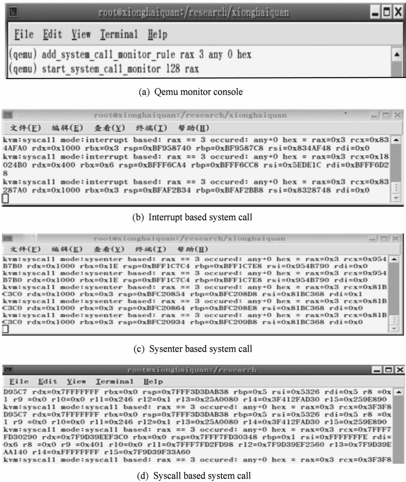
Fig. 16 Qemu monitor and the functional verification of three system call mechanisms interception and identification.
