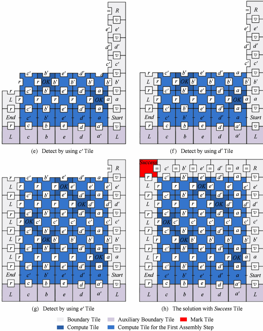
Fig. 4 Perfect matching self-assembly model of the bipartite graph G shown in Fig. 1.
