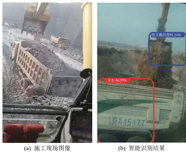
Fig. 4 Intelligent monitoring case of construction equipment based on vision
