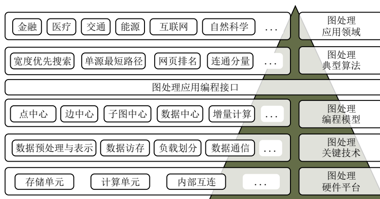
Fig. 1 The layer framework of graph processing system
