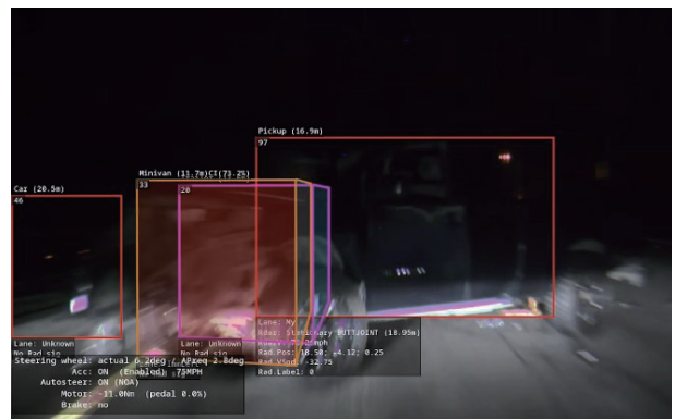
Fig. 15 Result diagram of the target detection system when the Tesla autonomous vehicle accident occurs
