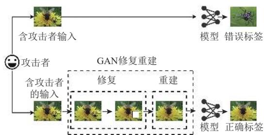
Fig. 8 Februus<sup>[18]</sup> reconstructs masked regions using GAN-based repair method
