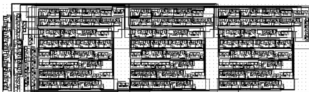
Fig. 15 The layout of 3 stages FIFO as synchronous-asynchronous interface.
