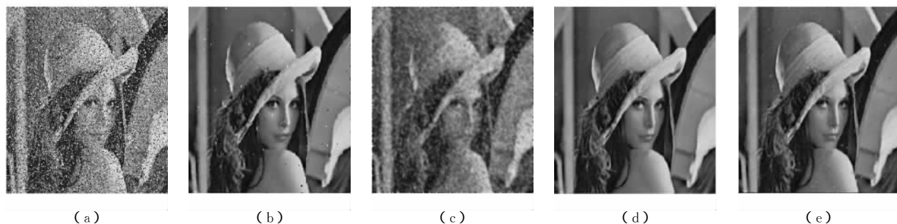
Fig. 5 Comparison of denoising on the Laplace noisy Lena image with variance of 25 under different variational models.
