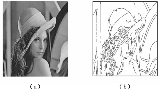
Fig. 3 Original Lena and ideal edge map. (a) The original Lena image and (b) The ideal edge map with 21220 edge pixels.
