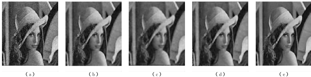
Fig. 4 Comparison of denoising on the Gaussian noisy Lena image with variance of 15 under different variational models.
